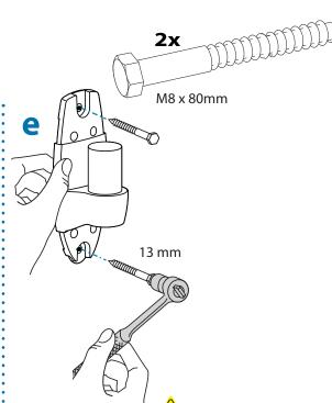
CAUTION: Make sure the wall mount bracket is level, flush and snug to the wall surface. DO NOT OVERTIGHTEN THE BOLTS.
