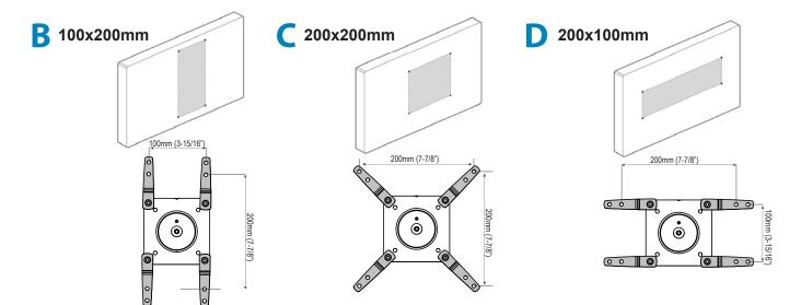
Mount VESA Adapters to Arm based on TV/Monitor hole pattern size (B, C, or D).
